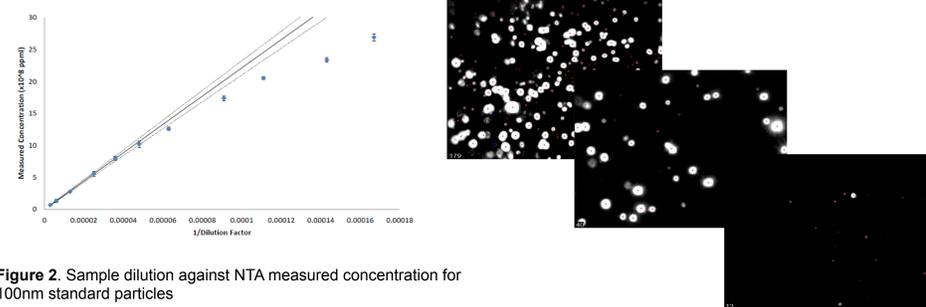
Figure 2. Sample dilution against NTA measured concentration for 100nm standard particles
