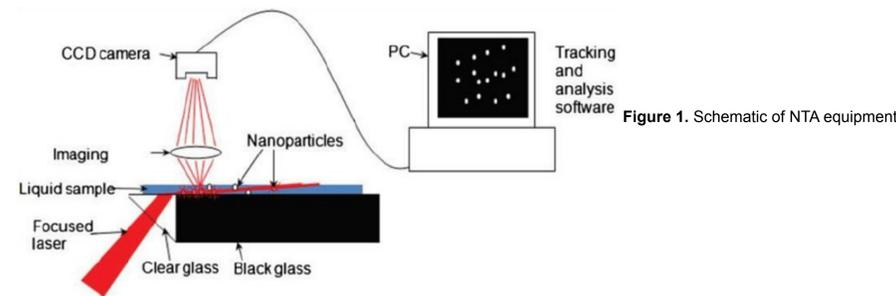
The particle-by-particle approach of NTA allows accurate measurement of particle concentration within a liquid suspension (particles per mL).
